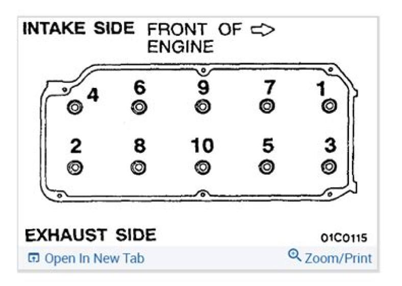
3. Tighten the bolts by the procedure shown in the illustrations.
