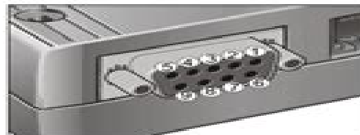
Figure 5: Pin assignment RS-232 (D-Sub 9-pole female)
