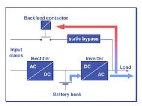
preventing feedback to the mains from the inverter in case of mains failure and a fault in the bypass circuit
