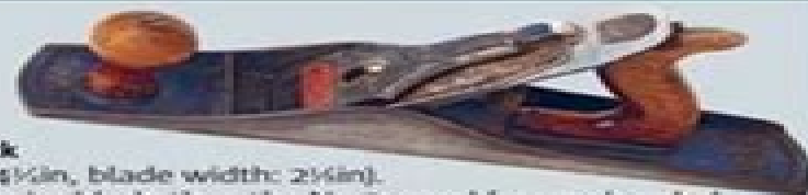
No.5 Jack (length: 14in, blade width: 2in). Good for a wide range of tasks, including some preparation.
