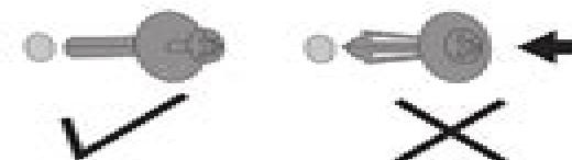
Do not push in the head of the fastener until you have inserted the fastener into the bracket and the hole on the TV. Do not use a screwdriver to tighten the screws.
