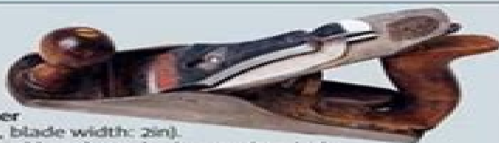
No.3 Smoother (length: 8in, blade width: 1½in). Lighter, more suitable for smaller hands.
