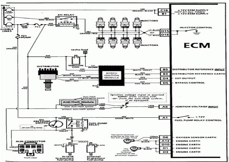
ECM Wiring (1 of 3): POWER & EARTHS, INJECTORS, IGNITION, FUEL PUMPS
