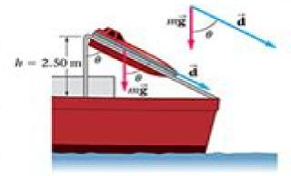
**Known** Mass of lifeboat, m = 4970 kg; sliding distance, d = 5.00 m; vertical height, h = 2.50 m. **Unknown** Work done by gravity, W = ?
