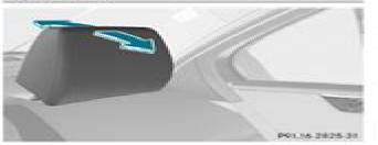
Adjust the head restraint to the desired position by pushing or pulling on the upper edge of the head restraint cushion.
