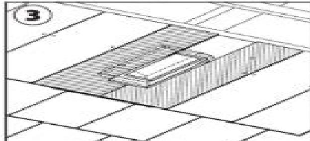
1. Lay slates to the required position of the ventilator. Cut the slate directly below the ventilator so that it does not protrude past the slate batten. Cut a 280mm wide gap in the batten at the head of the slate as shown.
