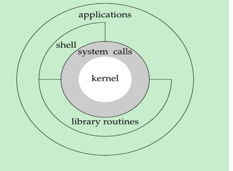
Figure 1.1 Architecture of the UNIX operating system
