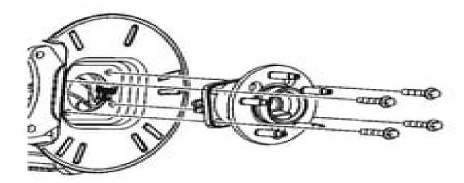
Fig. 1: Identifying Bearing Hub Courtesy of GENERAL MOTORS CORP.
