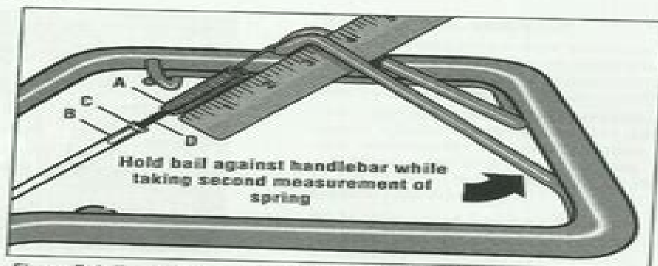
Figure 5-4: To check forward belt tension, take two measurements of the overall length of the coils in the spring – first with the clutch bail open, then with the clutch bail closed against the handlebar.
