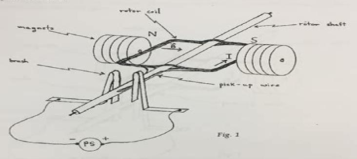
Pre-lab task #1: (1 point) Assume the rotor is in the position shown and the current in the rotor loop is as shown. If we replace the loop with a bar magnet having the same magnetic field, in what direction would the north magnetic pole of the bar magnet point?
