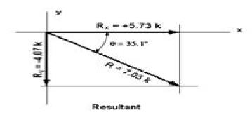
$$\begin{split} F_{1y} &= +F_1 \cos 30^\circ = 10k(0.866) = 8.66k \\ F_{1x} &= +F_1 \sin 30^\circ = 10k(0.50) = 5k \\ F_2 &= -F_{2x} = -12k \\ F_{3x} &= +\frac{1}{\sqrt{2}}(F_3) = +\frac{18k}{\sqrt{2}} \\ F_{3y} &= -\frac{1}{\sqrt{2}}(F_3) = -\frac{18k}{\sqrt{2}} \\ F_{3y} &= -\frac{1}{\sqrt{2}}(F_3) = -\frac{18k}{\sqrt{2}} \\ F_{3y} &= -\frac{1}{\sqrt{2}}(F_3) = -\frac{18k}{\sqrt{2}} \end{split}$$
