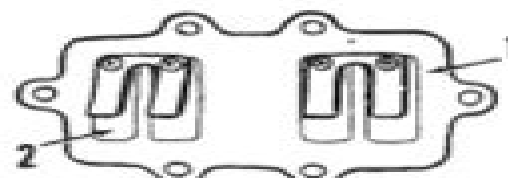
Fig. S24-4—View showing reed plate (1) and reed valve (2) assembly used on DT5 models.
