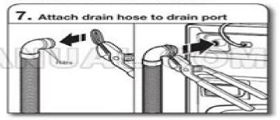
If clamp is not already in place on elbow end of drain hose, squeeze clamp with pliers and slide it over end of hose, centering it between the ribs, as shown. Squeeze clamp with pliers and slide elbow end of drain hose onto drain port and secure with clamp.
