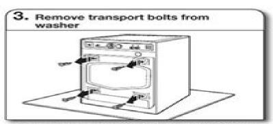
Loosen bolts with a 1/2" (13 mm) wrench. Slide each bolt and spacer to center of hole. Pull bolts and plastic spacers from back of washer. Discard bolts and spacers.
