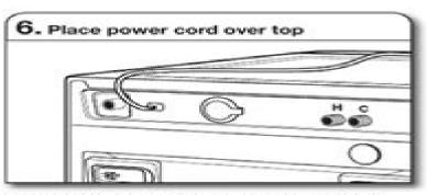
Remove the yellow shipping strap from the cord. Gently place power cord over top of washer to allow free access to back of washer.
