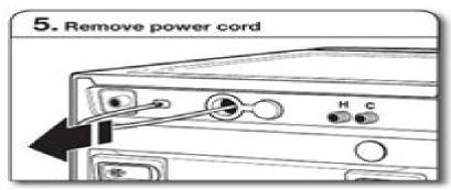
Pull power cord through opening in rear panel and close hole with attached cap.
