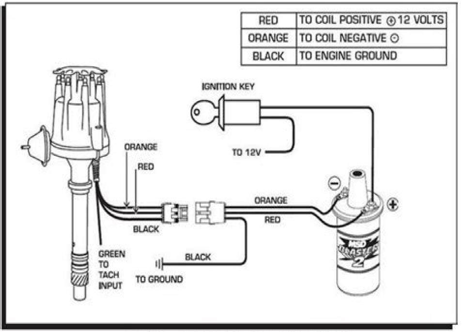
Figure 10 Wiring the Ready-to-Run Chevrolet Distributor.
