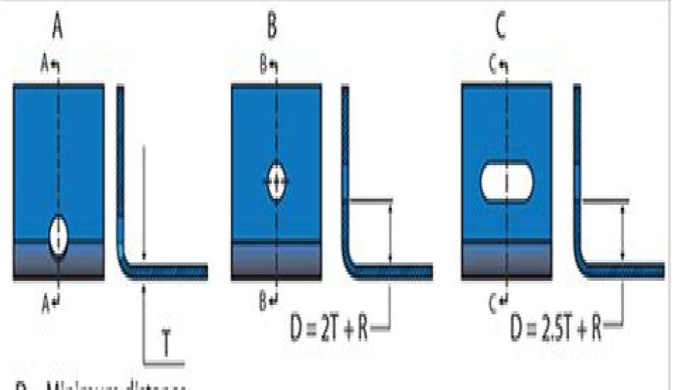
D = Minimum distance T = Material thickness R = Bend radius
