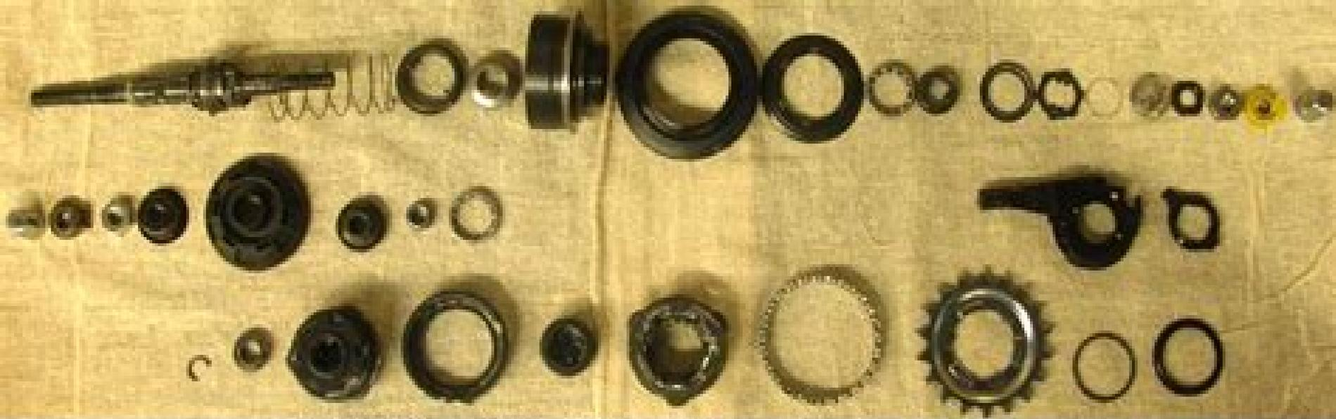
NEXUS 7-Speed Internal Hub w/Hi-Power Roller Brake
