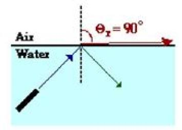
When the angle of incidence equal the critical angle, the angle of refraction is 90-degrees.
