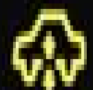
Air suspension warning
