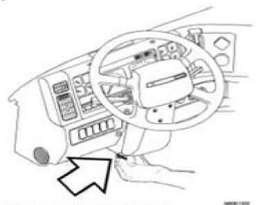
Remove the 2 clips at the bottom of the steering column cover. March Co.
