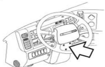
Remove the rear steering column oover by removing the 3 torx bolts from the cover and sliding the rubber M600-1500
