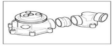
Press the intermediate pipe into the thermostat housing and coolant pump.
