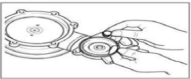
106. Fit the O-ring into the thermostat housing.
