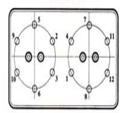
Torque cylinder head nuts following illustrated sequence when the intake/exhausts manifolds are in place to insure proper alignment. ENGINE MUST BE COLD FOR THIS PROCEDURE. Use a cross-sequence for tightening the nuts. Consider both cylinders as one unit because they are joined by exhaust and intake manifolds. Torque spec for cylinder head nuts (8mm) = 22NM/195 in lb. Requires 13mm socket.
