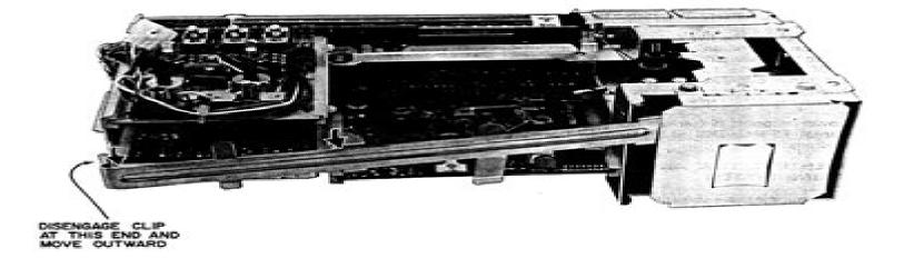
FIGURE 7 - RETAINING BRACKET REMOVAL
