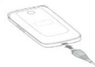
Connect the charger to a standard AC wall outlet. If the phone is on, you'll see a charging icon, such as E or N, appear in the Status Bar.
