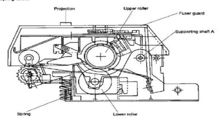
\*2 When the upper unit is open, the upper roller is pushed up by the spring force, and only the weight of the upper roller itself is applied to the lower roller.
