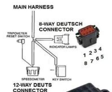
a. CONNECT TO PINK WIRE LOCATED AT SPEEDOMETER CONNECTOR (IS TAPED BACK TO WIRE HARNESS)
