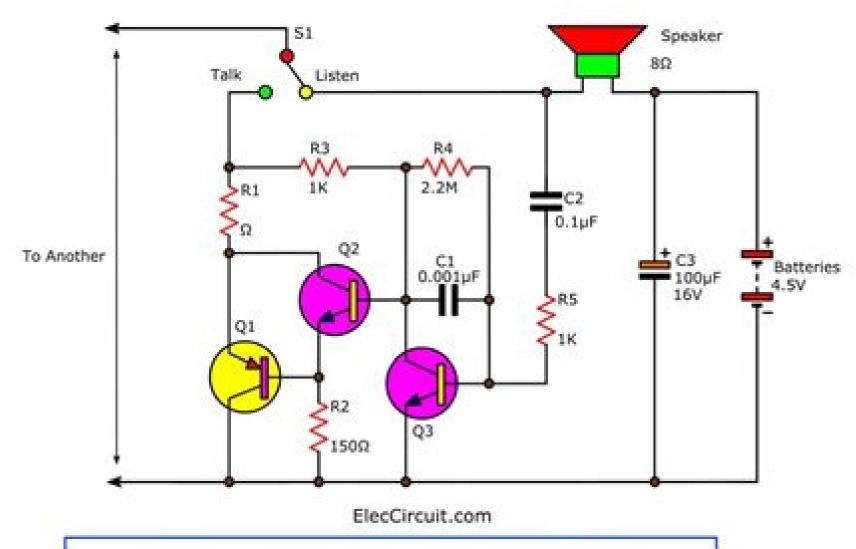
Transistors Intercom Circuit
