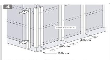
Fix cladding battens; Use double battens at corners, edges and junctions. Refer to Diagrams 7 & 8 before cutting battens to length.
