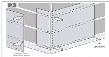
Affix breather membrane to cover entire surface to be clad. (Ensure membrane is lapped according to manufacturer's instructions)
