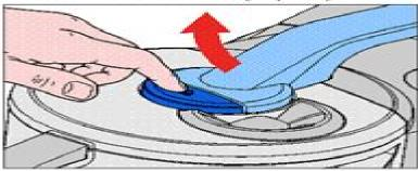
The button (3) on the lid is a spare part, it can be replaced by removing screw (see picture).
