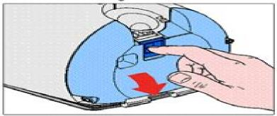
To reach the inner parts for repair, Upperhousing (18) has to be removed. First the On/Off button (17) and Cordwinder button (16) must be removed, this can be done with a screwdriver (see picture).
