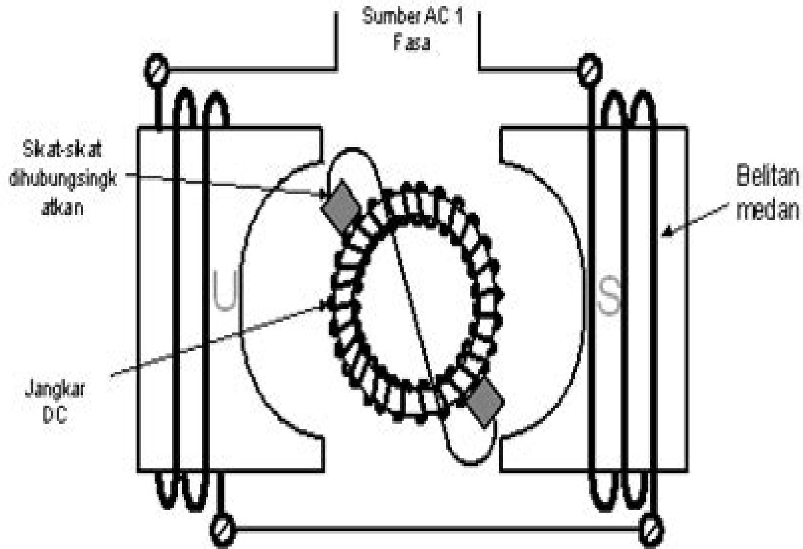
Gambar 06. Sirkuit diagram motor repulsi
