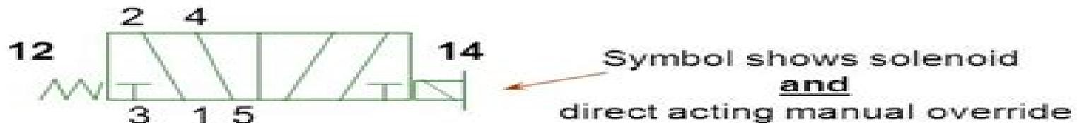
**NOTE:** Flow path arrows omitted to show multi purpose nature of valve. How the valve is piped will determine flow paths.
