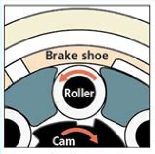
Cam and roller rotate when brake is applied.
