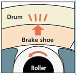
Brake shoe contacts drum to begin braking.
