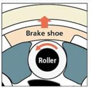
Brake shoe moves up to drum while roller is rotating.
