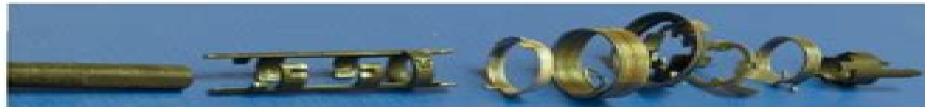
Figure 2. Axle unit parts as in an exploded view.
