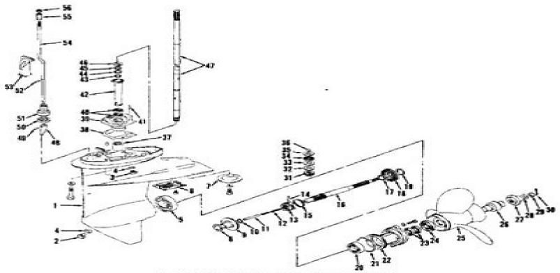
Fig. 527-22 - Exploded view of lower unit go
