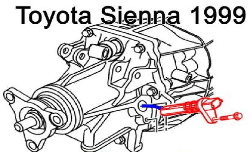
My Speed Sensor (Red) has a wire (Blue) that runs into the transmition. And I never see that in any diagrams or YouTube how-to-videos. I don't know how to replace my speed sensor because it attached this wire.
