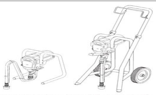
This pump is available in a stand model (9140S) and cart models (9146. 9150, 9170 and 9190). All information given for the stand model applies to the cart models except where indicated.
