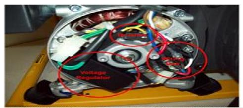
Under the cover you will see the main components of the generator circuit. The Voltage Regulator is a rectangular box held in place with two 7mm screws.
