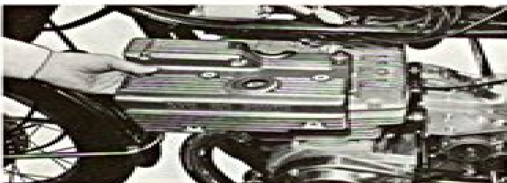
Fig. 7-1-21 Removing cylinder head covers
