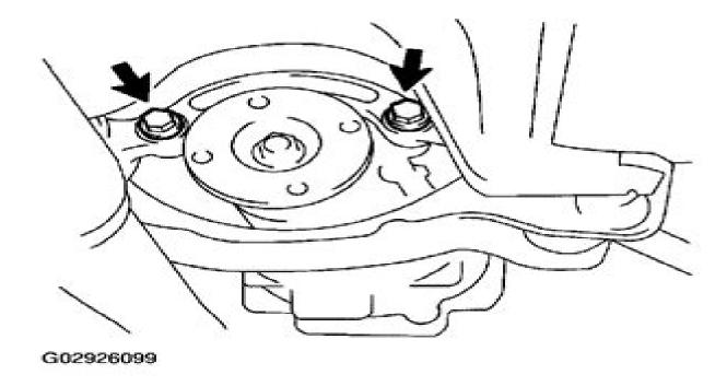
Fig. 5: Removing Differential Rear Mount Cushion & Bolts Courtesy of TOYOTA MOTOR SALES, U.S.A., INC.
