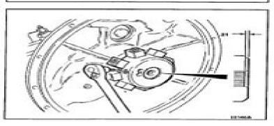
The main hydraulic pump (1) is mounted directly to the engine flywheel housing with twelve hex head bolts. Torque to 35-40 lb. ft. (47-54 Nm).
