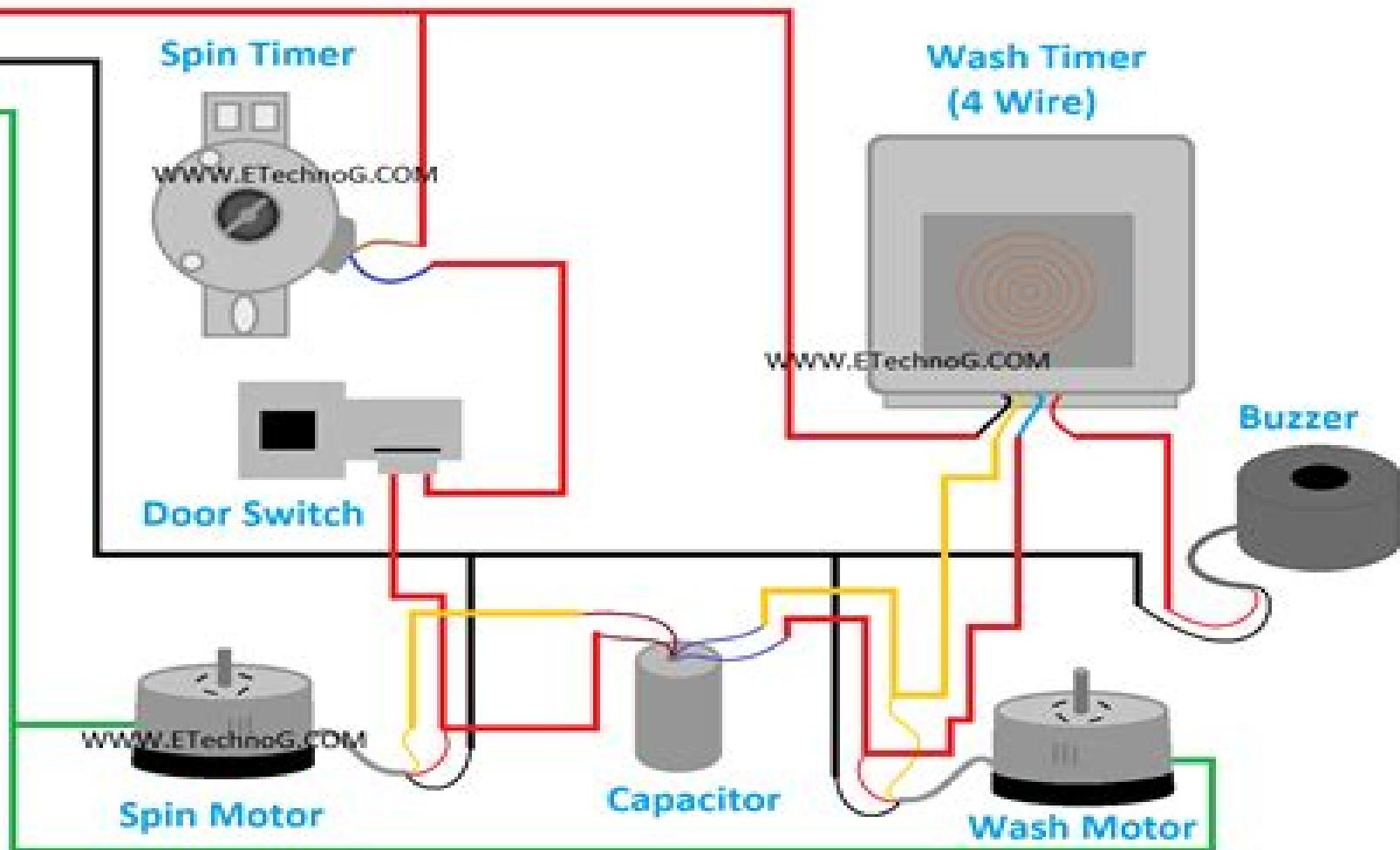
**Washing Machine Wiring and Connection Diagram**
