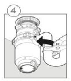
Make all connections, plug in disposal and test for leaks
