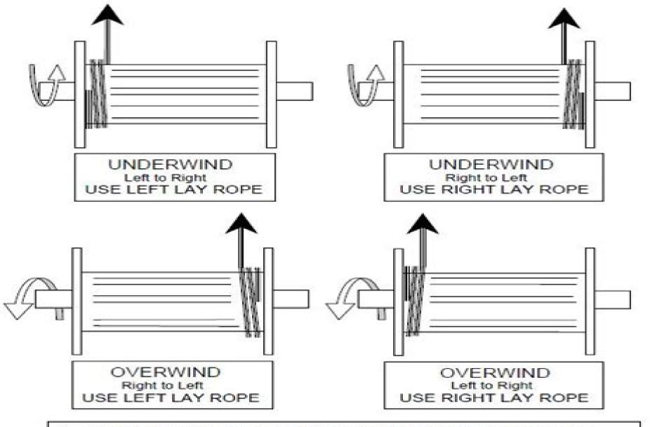
If a winch is aligned and cable still keeps piling up on one part of the drum the problem could be that the wrong cable is being used. Willard Says.....Wire Rope tells how to identify different styles of wire rope. The above sketches show various winch arrangements with the recommended style of wire rope for each.
