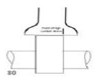
The whole procedure exerts an enormous strain on the components involved, sometimes 'stacking-up' contact stresses over the cam nose as high as 1300 Meganewtons/sq m. (200 lbs/sq in.), calling for a high degree of accuracy in design and manufacture, together with the need for great care and attention when fitting
