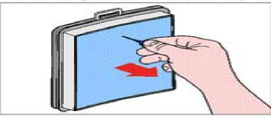
The bottom of the Bucket can be removed as shown in the picture below.
