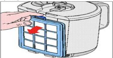
The foam in the Inlet filter assy can be cleaned.
