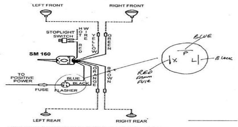
NOTE: To ensure proper grounding of switch, scrap or sand a small area of point from steering column under the clamp to allow bare metal contact.
