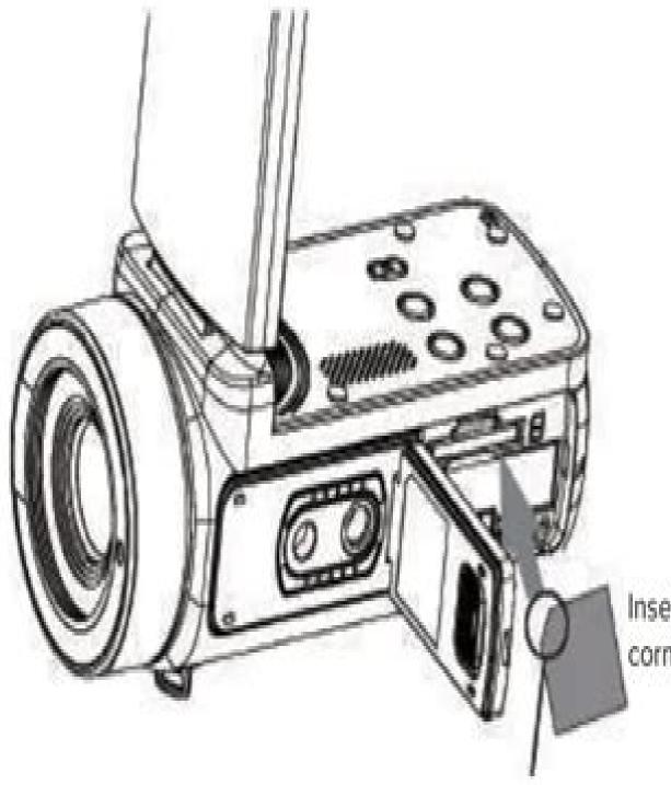
Insert the card with the noted corner in the direction as illusrated.
